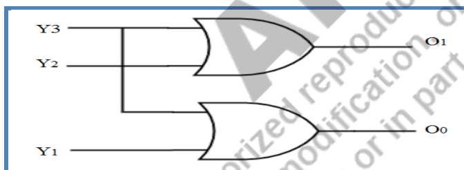
Fig. 3.14: Logic Circuit of 4:2 encoder
