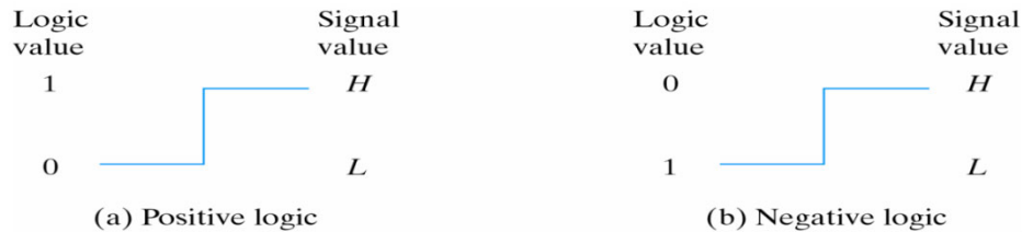
Figure 2.2(a) Positive logic (b) Negative logic
